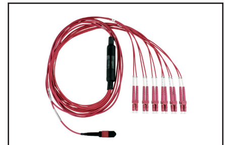
FP4LDMF002M, FX Hydra Patch Cord, OM4, MPO-12F (F) to 6 x LC Duplex, 2 m
